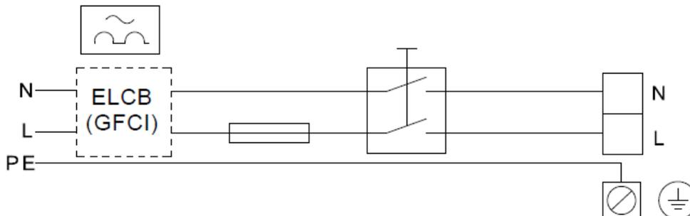
The mains connection to the pump should be via a suitably rated isolator/switch. Cables should be 1.5mm<sup>2</sup> and backup fuses rated at 10A. The mains supply should enter the panel via the cable gland provided.
