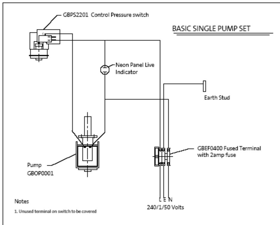
The unit should be connected to a single phase 220-240V supply as shown in the diagram above. The three core cable should be brought into the unit via the mains cable gland supplied and the unit is internally fused with a 2A fuse.
