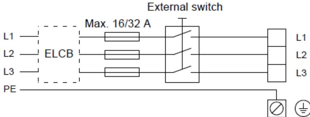
The mains connection to the pump should be via a suitably rated isolator/switch. Cables should be 1.5mm<sup>2</sup> and backup fuses rated at 16A and the mains supply should enter the panel via the M20 cable gland provided. Three phase cables plus an earth are required (no neutral wire).
